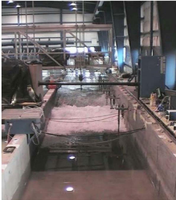
**Figure 7 Breaking bore**
