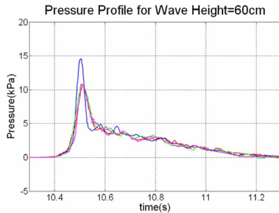
**Figure 11: Uplift pressure on floor slab for bores caused by 20, 40 and 60 cm solitary waves with no water on reef**
