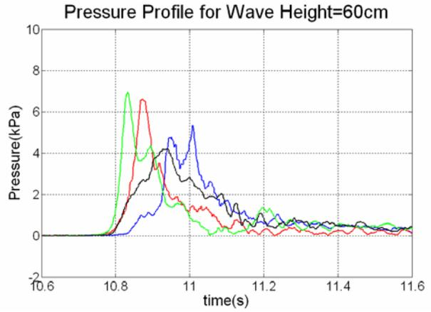
Figure 12: Uplift pressure on floor slab for bores caused by 20, 40 and 60 cm solitary waves with 10 cm water on reef
