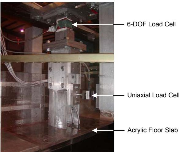
Figure 7: Details of floor slab instrumentation
