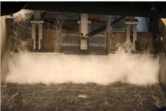
Figure 8: Bore impact on wall and floor test configuration
