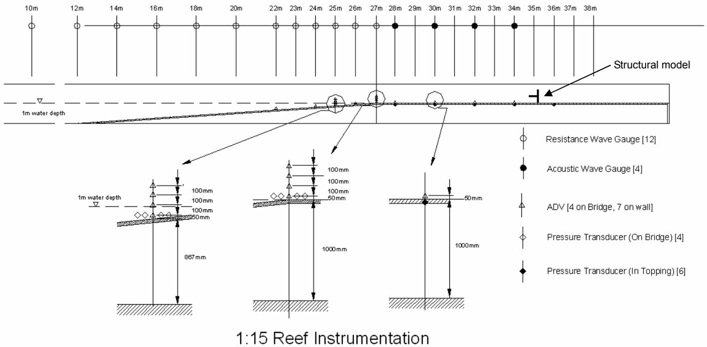
**Figure 5 Beach slope and fringing reef with instrumentation**
