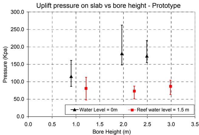
Figure 14: Prototype uplift pressure vs. bore height
