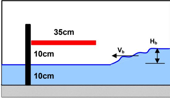
Wall-slab test configuration with incoming bore
