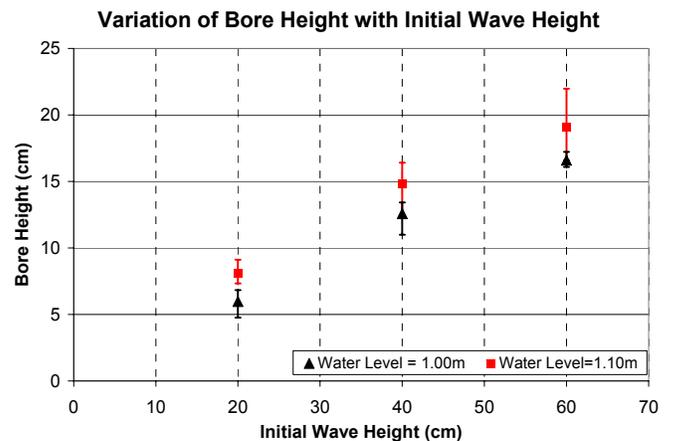
Figure 9: Variation of bore height with initial wave height
