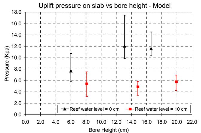
**Figure 13: Model uplift pressure vs. bore height**
