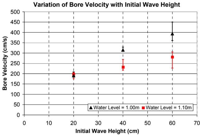
**Figure 10: Variation of bore velocity with wave height**
